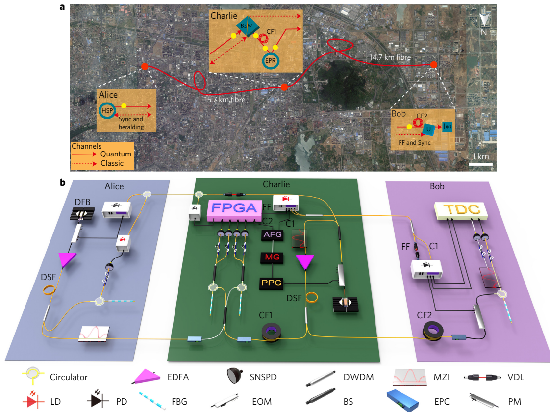
Figure 2 | Quantum teleportation in a Hefei optical fibre network. a , Bird's-eye view of the experiment. Alice prepares the quantum state, |\psi\rangle_{in} , on a heralded single photon (HSP) and sends it to Charlie, who shares an EPR pair with Bob beforehand. Each photon of the EPR pair is stored in a 15 km coiled optical fibre (CF). Charlie implements a BSM on his photon and the received HSP and then sends the feedforward signal to Bob, who performs a unitary correction operation (U) and state analysis. The quantum signals are transmitted in the optical fibre denoted by the solid line, whereas the classical signals are sent in another optical fibre denoted by the dashed line. b , Experimental set-up. Both Alice and Charlie generate photon pairs through the FWM process in the DSF. The MZIs are used in the state preparation and measurement (Methods). The microwave generator (MG) serves as master clock. To synchronize (Sync) the HSP source and EPR source, Charlie sends a portion of his pulse laser beam to Alice through an optical fibre channel, and Alice detects them by using a 45 GHz PD to generate driving pulses for an EOM. The heralding signals are converted into a laser pulses with a laser diode (LD) and transmitted to Charlie through the same optical fibre. Two optical circulators are used to achieve the bi-direction signal transmission. The feedforward signal (FF) and clock signals (C1, 10 MHz clock signal and C2, 200 MHz clock signal) generated by the arbitrary function generator (AFG) are carried by laser pulses with different wavelengths, which are launched into an optical fibre by a DWDM filter and sent to Bob. After being separated by another DWDM, the feedforward signal and 10 MHz clock are converted into electrical signals and fed to a time-to-digital converter (TDC). The feedforward signal is also used to trigger a short PG module to generate the driving pulse for the phase modulator (PM) to perform the unitary correction operation. Electronic-controlled polarization controllers (EPC) are used to compensate automatically the polarization drift caused by the optical fibre. Map data: Google. CNES/Astrium. DigitalGlobe.
